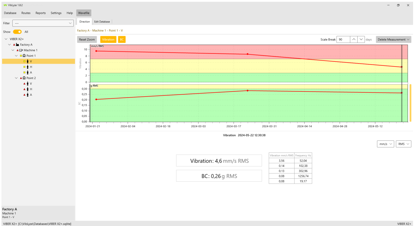
Trend graph in VibLyze displaying vibration data from VIBER X2+
