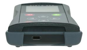
**USB-C connector** Used to connect the VIBER X2+ to a PC for transfering files or connecting to a charger to charge the battery.
